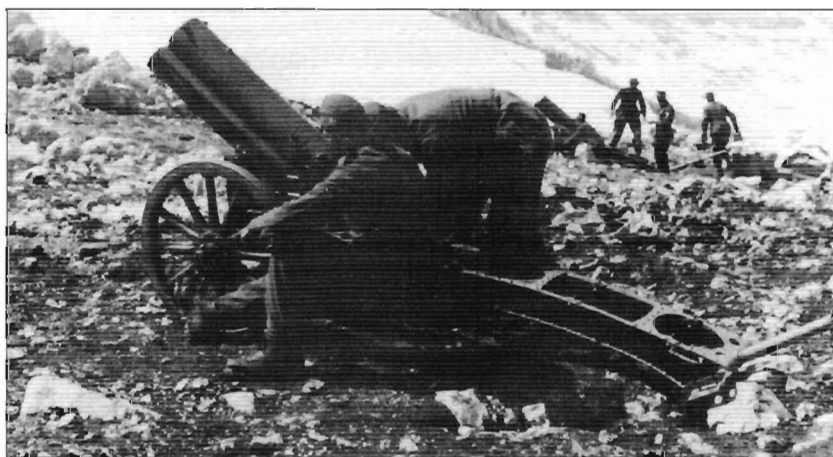
A Gebirgsjäger Abfeuren-Batterie with a pair of the obsolescent Skoda 7.5cm GebK15 mountain guns which were first issued to Bruno Schram's Artillerie-Versuchszug. That they were hardly suitable for the airborne role is obvious.
